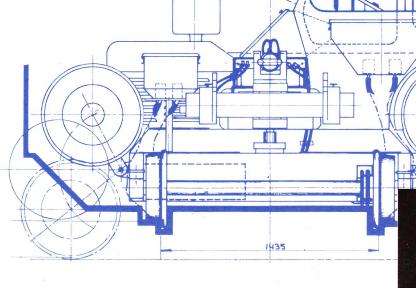
The industrial locomotive that never lets you down: Trackmobile. A highly sophisticated system allows Trackmobile to move on rails as well as on the road. It's the last word in ease-of-use and efficiency. In addition, due attention has been given to the driver's safety. All coupling operations are carried out from the driver's cabin. The Trackmobile series has recently been expanded with a heavier duty model – the 45 TMC.
